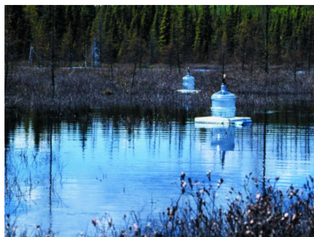
Figure 2. A static floating chamber deployed in the backwaters of the Experimental Lakes Area Reservoir Project reservoir. Fluxes of \text{CO}_2 and \text{CH}_4 from the surface of the reservoir are calculated by measuring the rate of buildup of these gases over time inside the chamber. Photo courtesy of V. L. St. Louis.
